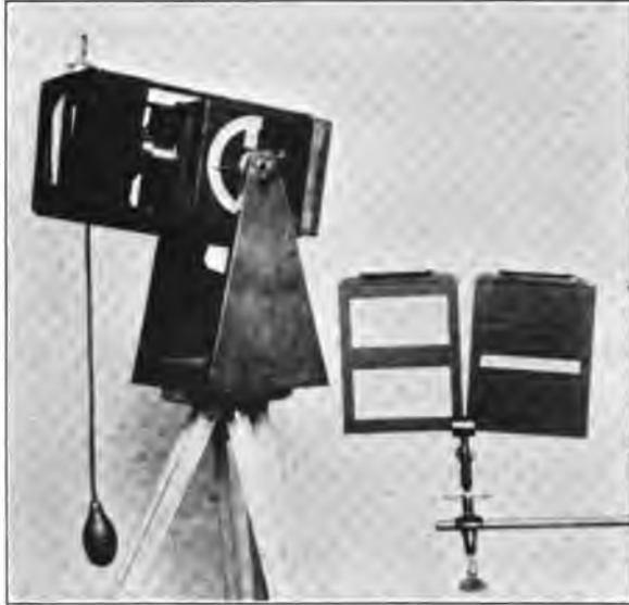
Fig. 55 — Apparatus for studying the distribution of brightness in Nature.
